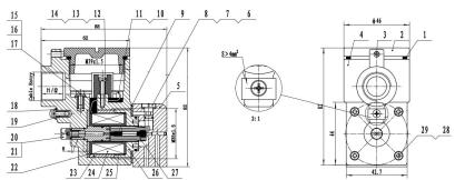
6.2.4 Electrical connection is made with junction box with M20-1.5 or 1/2" cable entry, two points terminal strip for electric pins + ground pins and outside ground pins is available.
